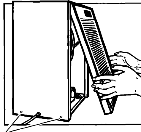
SOCKET-HEAD SCREWS (SIDES OF CABINET)
